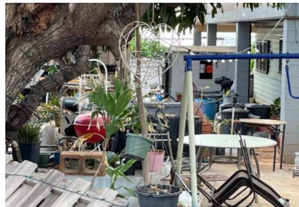
Figure 2.8b. Example of hazardous defensible space with excessive storage of combustibles within Zone 0 (0-5 ft) and Zone 1 (50-30 ft). Image courtesy of Jensen Hughes/FEMA.
