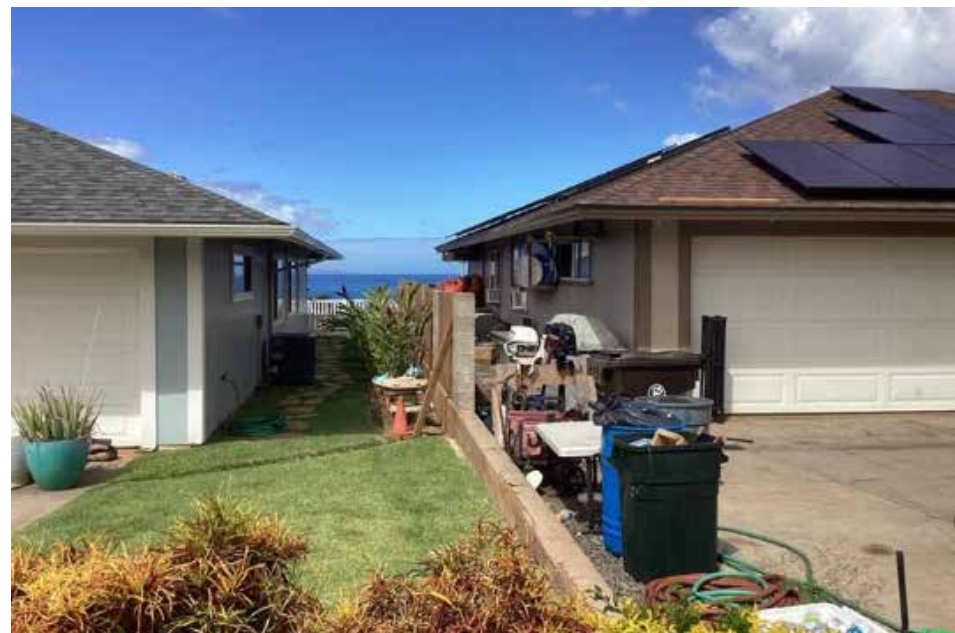
Figure 2.14. Example of closely spaced homes with home on right having hazardous amounts of combustibles stored in Zone 0 (0-5 ft). This presents an increased fuel / fire hazard to both homes. Image courtesy of Jensen Hughes/FEMA.
