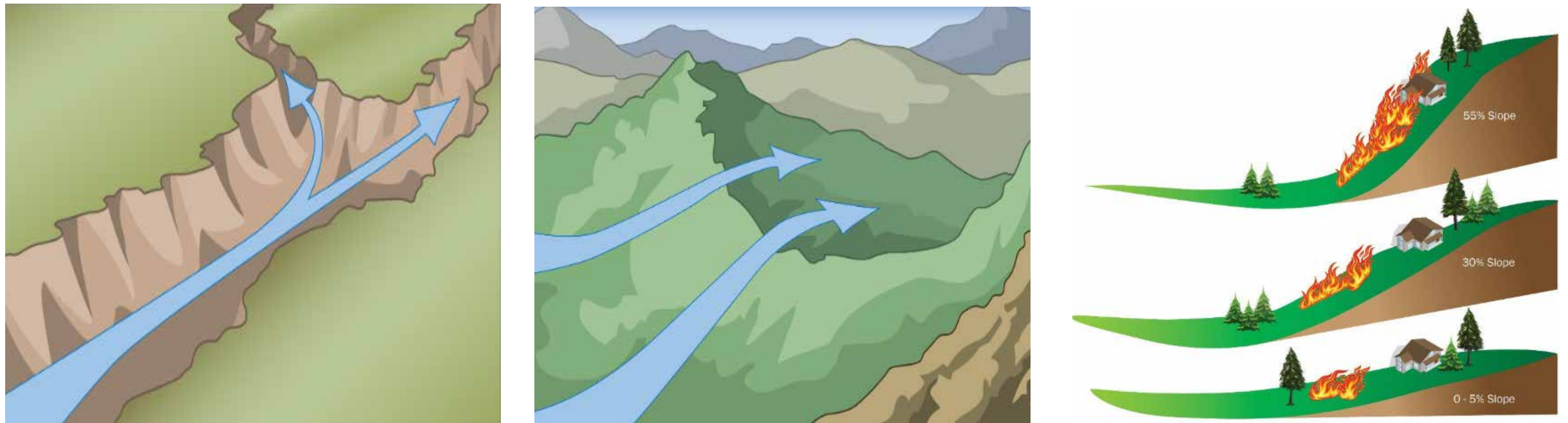
Figure 3.4. Common topographic fire hazards. (left) Canyons can collect heat and funnel superheated air. (middle) Winds are funneled over a saddle between two peaks. Images adapted from Home Builder's Guide to Construction in Wild-fire Zones, FEMA, 2008. https://www.fema.gov/ (right) The steepness of the slope can impact fire spread. Image adapted from FEMA Marshall Fire MAT, Best Practices for Wildfire Resilient Subdivision Planning, FEMA, 2023. https://www.fema.gov/
