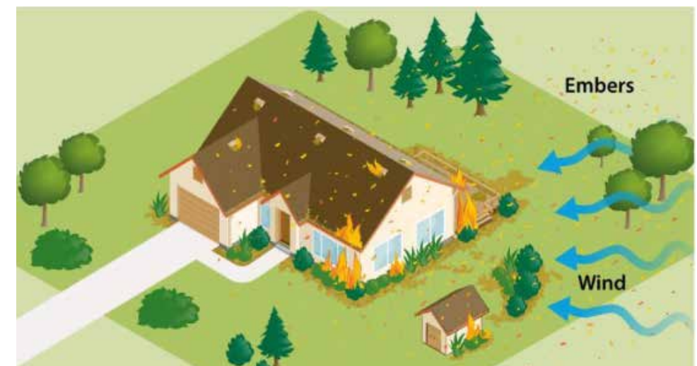
Figure 2.6. Three main heat transfer mechanisms that lead to structure ignition: (1) direct flaming contact, (2) radiant heat, (3) embers or firebrands. Reprinted from UC ANR Publication 8695, CC BY-NC-ND 4.0.
