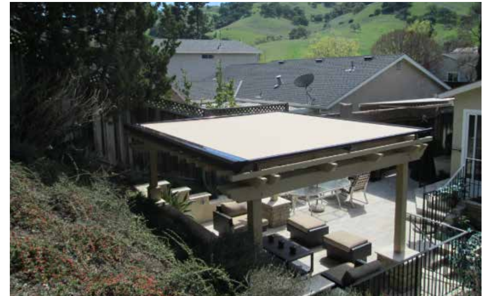
Figure 1.83. Example of retractable pergola cover. If the cover is made of combustible material, this cover can ignite and pose an exposure hazard to the home. Image by European Rolling Shutters, CC BY 2.0.
