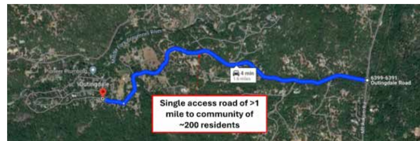
Figure 3.11. Example of single access/egress route for a residential neighborhood. During a major wildfire, the single point of access/egress could be blocked by the fire incident (e.g., severe conditions, downed trees, car breakdown), potentially trapping or exposing a large number of people to untenable conditions, as well as limiting effective access by first responders. Image courtesy of Jensen Hughes/FEMA.
