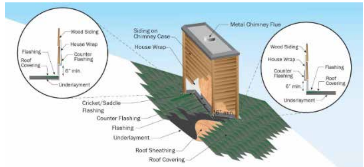
Figure 1.23. Sample flashing details at chimney-to-roof joint. Note: Flashing shown in this figure is intended to be non-corrosive, metal flashing. Image adapted from FEMA Marshall Fire MAT, Wildfire Resilient Detailing, Joint Systems, and Interfaces of Residential Building Components, FEMA, 2023. https://www.fema.gov/
