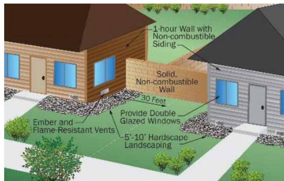
Figure 2.15. Sample mitigations where site constraints limit setbacks to less than 30 feet. A combination of enhanced structural hardening measures (e.g., 1-hour exterior fire walls, non-combustible, solid fencing, reducing # of windows) and enhanced defensible space measures (e.g., hardscaping extended to 10 feet). Image adapted from FEMA Marshall Fire MAT, Wildfire Resilient Detailing, Joint Systems, and Interfaces of Residential Building Components, FEMA, 2023. https://www.fema.gov/ .
