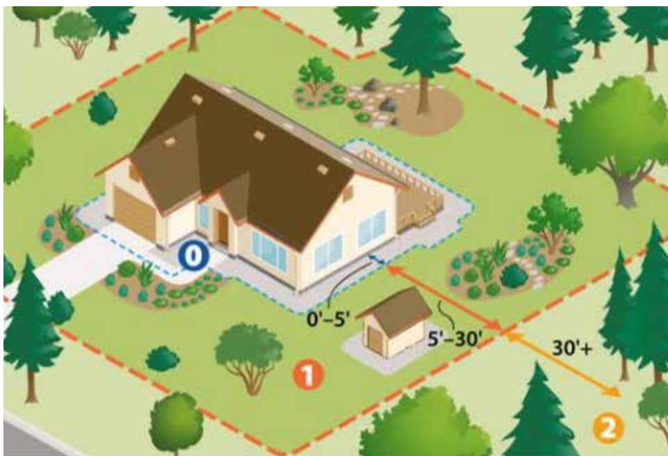
Figure 2.7. Reducing vegetative and man-made fuels around a structure are essential to reduce fire pathways from travelling to a property/structure, while also providing a safer place for firefighting operations. Reprinted from UC ANR Publication 8695, CC BY-NC-ND 4.0.
