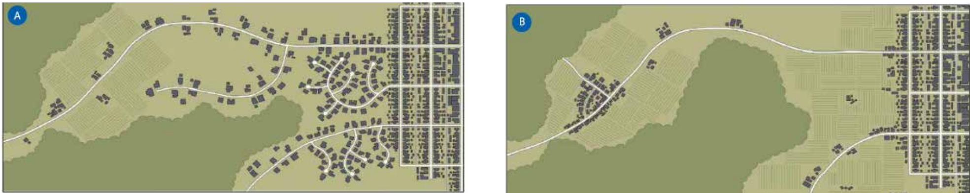
Figure 3.8. Conventional, or traditional, development with low-density houses (A) versus clustered development with several high-density clusters of structures (B). Image reprinted with permission from Martin Dreiling, Dreiling Terrones Architecture and the Smart Code.
