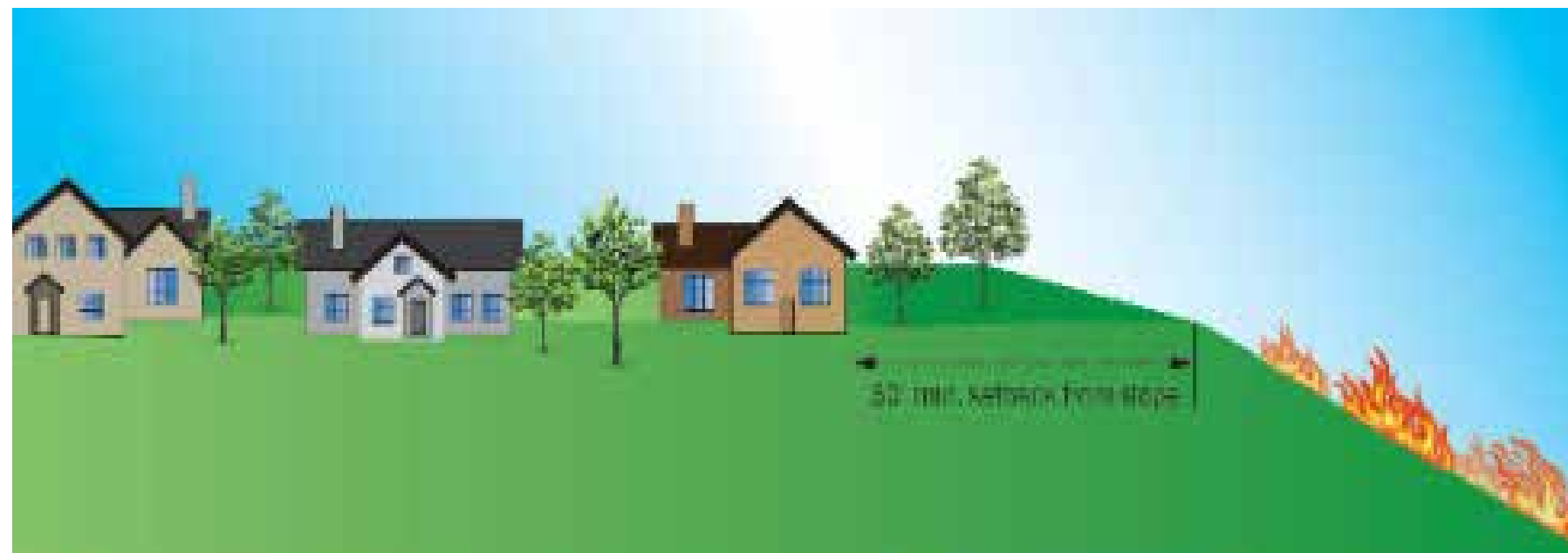
Figure 3.5. Developments located on or proximate to slopes >30% may have increased wildfire risk. Appropriate mitigation actions, such as slope setbacks, vegetation management plans and/or enhanced structural hardening may be needed to offset the increased wildfire risk. Image adapted from FEMA Marshall Fire MAT, Best Practices for Wildfire Resilient Subdivision Planning, FEMA, 2023. https://www.fema.gov/
