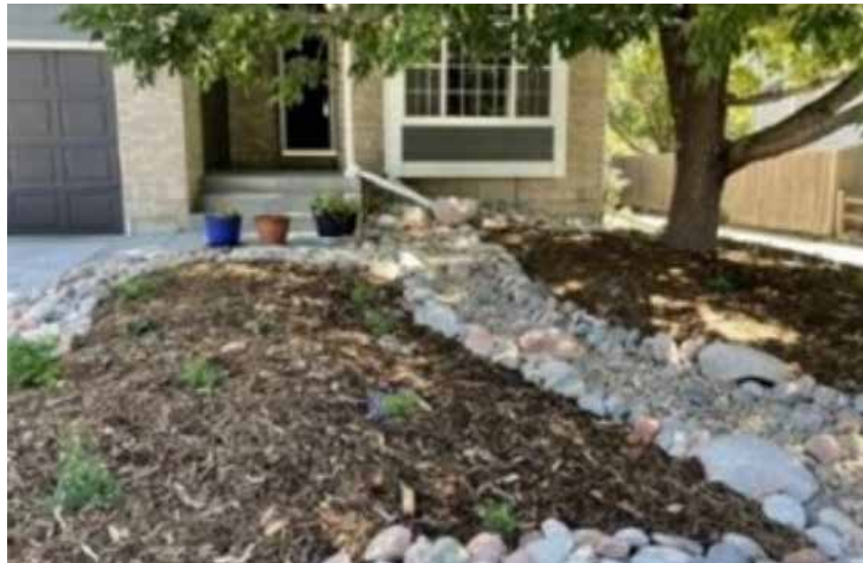
Figure 2.8c. Examples of hazardous defensible space with combustible mulch within Zone 0 (0-5 ft). Image courtesy of Jensen Hughes/FEMA.
