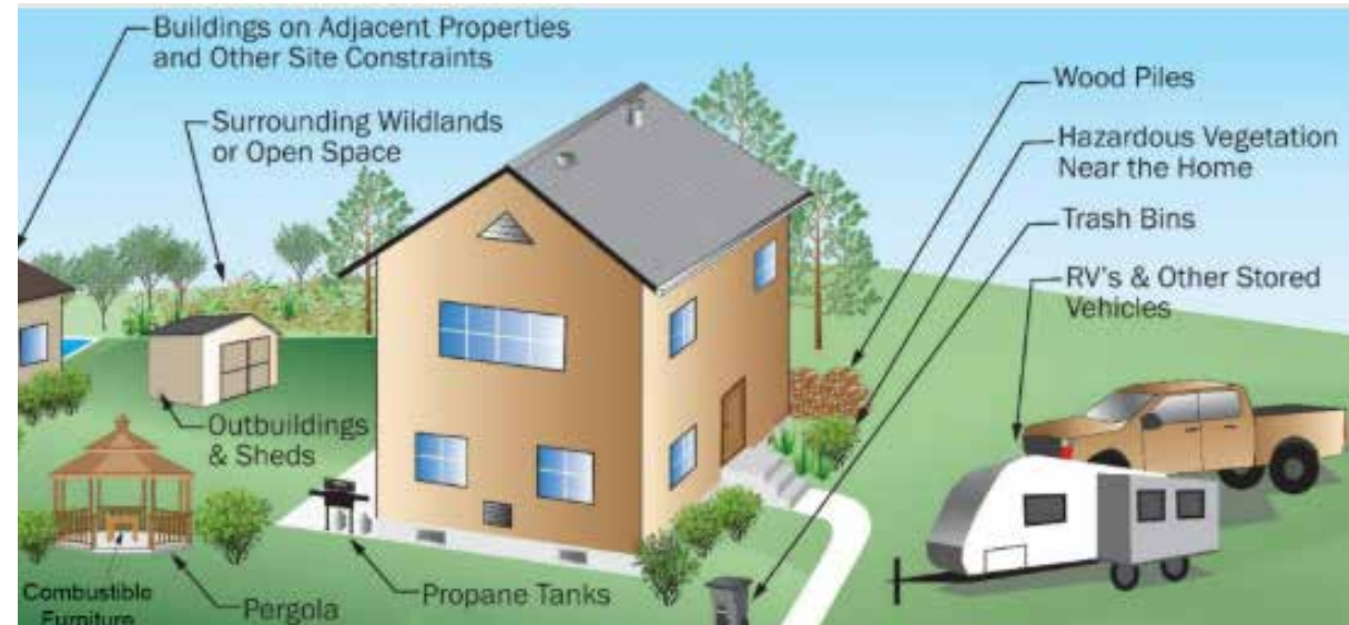
Figure 2.4. Variety of vegetative and man-made fuels surrounding a structure that are considered part of defensible space. Please note the furniture and pergola are combustible. Also note, the propane tanks and hazardous vegetation are within the closest zone and therefore too close to the structure. Credit: Image annotated by SFPE Foundation. Original diagram from FEMA Marshall Fire MAT, FEMA, 2023. https://www.fema.gov/
