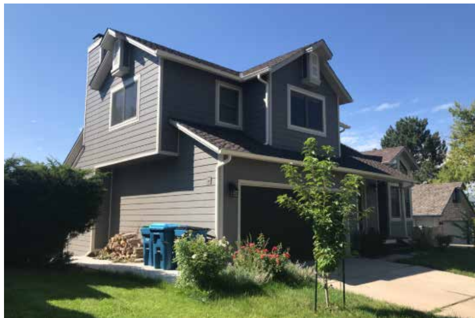
Figure 2.8d. Examples of hazardous defensible space with pile of firewood and plastic trash bins within Zone 0 (0-5 feet), heavy brush within Zone 1 (5-30 feet). Image courtesy of Jensen Hughes/FEMA.
